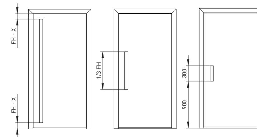
Depending on whether the casement design is flush or protruding, the corresponding bar handle is chosen. They differ with respect to their installation depth:
